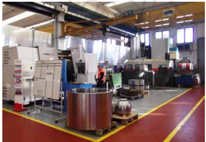
Horizontal (foreground) and vertical (background) lathes
