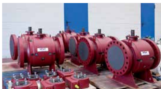
Valves in packing area after being tested
