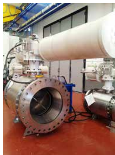
30" (750 mm) Class 300 actuated control ball valve with anti cavitation trim
