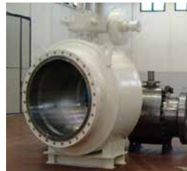
48" (1200 mm) class 300 ball valve for subsea service
