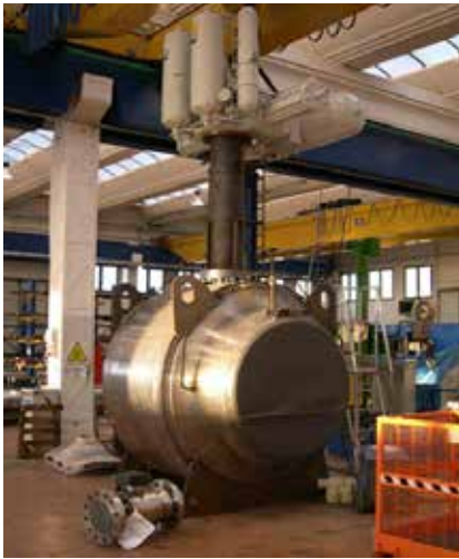
56" (1400 mm) Fully Welded, Class 600 valve
