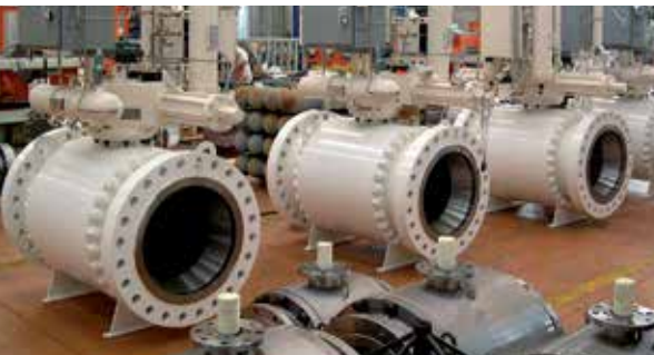
Actuated valves for testing in the in-house valve automation centre
